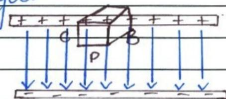
The electric field is directed from positive to negative plate. To find electric intensity, consider a gaussian surface in the form of a box in between the plates. The top of the box is in the positive plate.
