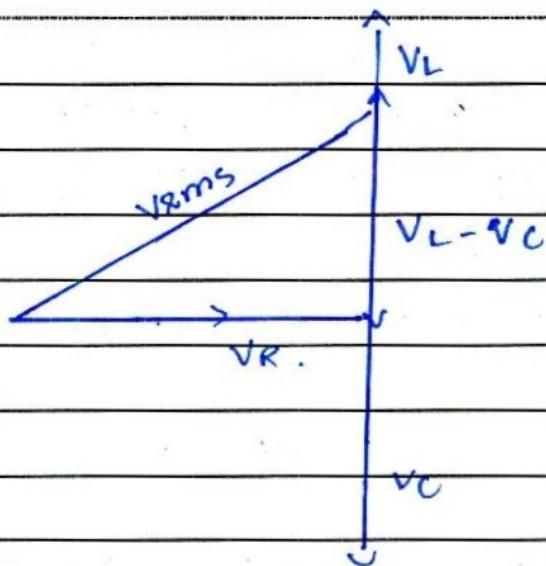
$$V_{rms} = \sqrt{V_R^2 + (V_L - V_C)^2}$$
