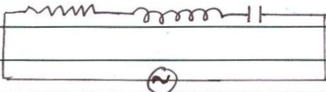
In a resistor current and voltage are in phase.
