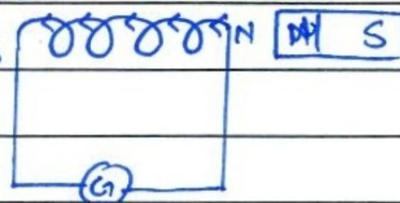
an e.m.f. current is induced. It opposes its cause and flows in anticlockwise direction.
