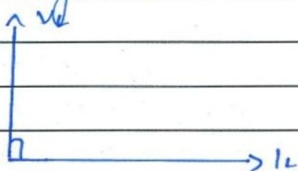
In a capacitor, voltage lags by  $90^\circ$ .
