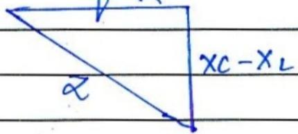
When  $X_L > X_C$ , circuit behaves as RL series circuit.
