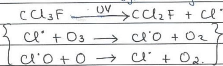
Net Reaction :-  $\text{O} + \text{O}_3 \rightarrow 2\text{O}_2$ .
