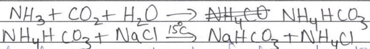
In the lower compartments of the carbonating tower, the temperature is lowered to  $15^\circ\text{C}$ . At this temperature,  $\text{NaHCO}_3$  precipitates out.
