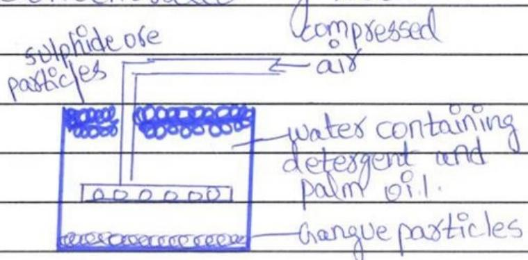
⇒ Diagram showing the concentration of sulphide ore:-
