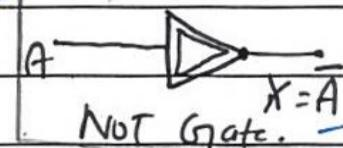
Inverter: NOT gate is called inverter because its basic function is inversion or complementation. It changes one logic level into opposite logic level. It inverts the state of Boolean variable.
